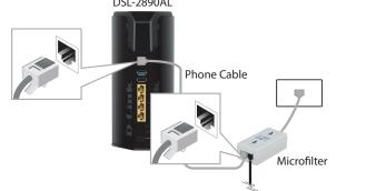
Connect the Ethernet cable from Ethernet port on your computer. Connect the Ethernet cable from the LAN port of the modem router to the
