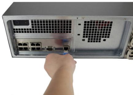
**Note:** The management port of the DSN-series does not support MDI and will require a crossover cable. Or if you wish, two standard straightthrough cables may be used with an intermediate switch or hub. The management port is 100MbE.
