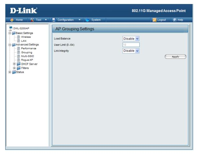
Load Balance: Load Balancing allows you to balance and share the wireless
