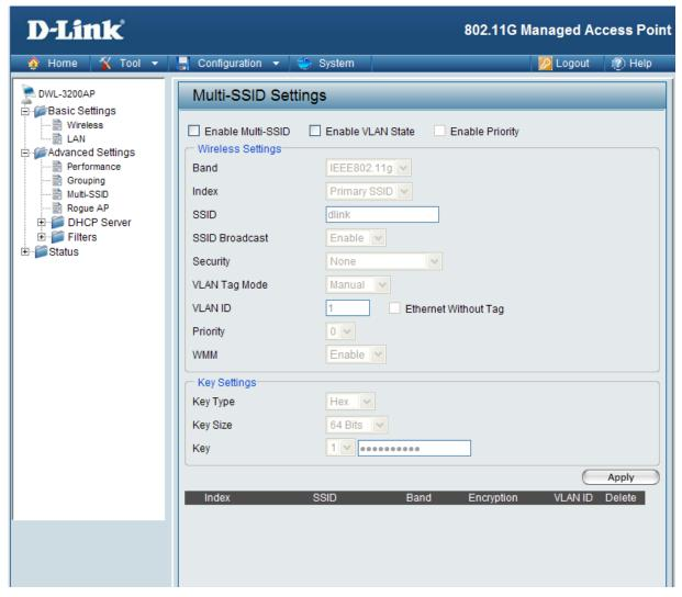
If you want to configure the Guest and Internal networks on Virtual LAN (VLANs), the switch and DHCP server you are using must support VLANs. As a prerequisite step, configure a port on the switch for handling VLAN tagged packets as described in the IEEE802.1Q standard.
