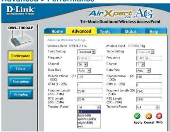
Wireless Band: Select 802.11a (up to 72 Mbps speed in turbo mode in the 5GHz range) or 802.11g (up to 54 Mbps speed with AirPlus adapters.)
