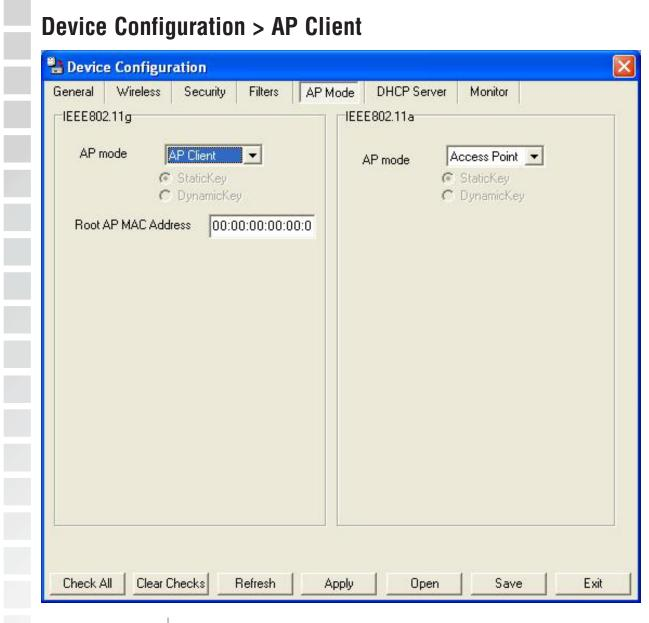
AP Client: In AP Client mode, the DWL-7700AP can be used as a client of a DWL-2700AP or another DWL-7700AP. Enter the Root AP MAC address of the DWL-7700AP that is acting as an access point in the network.
