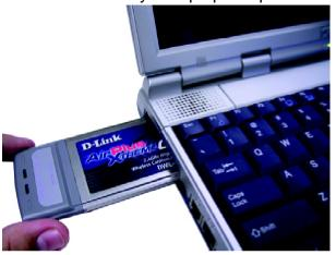
C. Gently insert the DWL-G650+ into the Cardbus slot in your laptop computer (as shown.)
