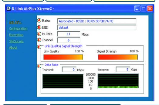
D. Channel: Displays the channel information. By default, the channel is set to 6 and selection is automatically determined by the DWL-G650+.
