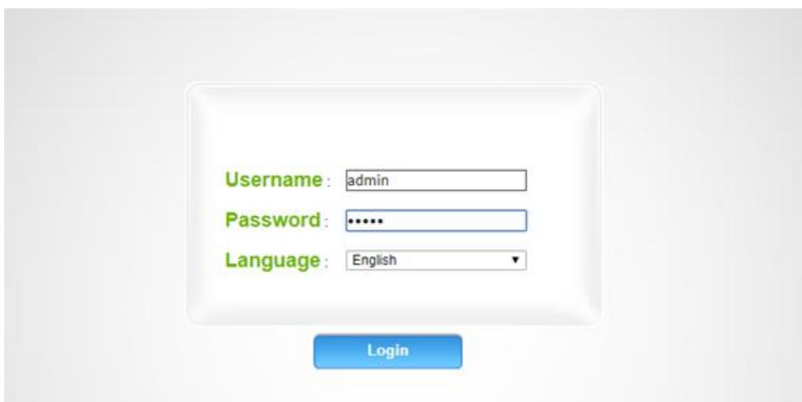
*If you cannot recall the password you have assigned to your modem, you will need to reset the modem to factory defaults by pressing the reset button for 10 seconds. Please note that this will revert all the settings in the modem to factory settings and you will have to reconfigure it with your Internet settings and Wireless security. Make sure you have your Internet account details (given by your Internet Provider) handy.*
