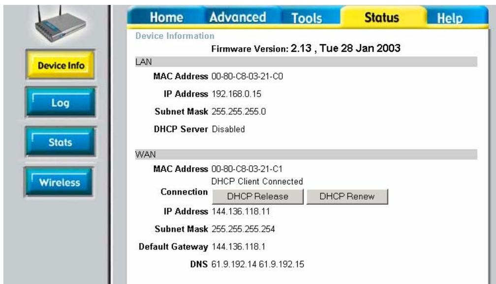
13. Now that the router setup is complete we now need to connect to Telstra via BPA Login. This is done by opening up the BPA Login program that we minimised earlier and clicking on the "Connect" button.
