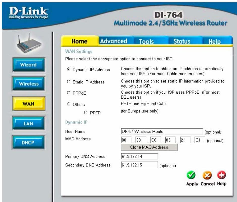
10. One thing of recent that is vital is the cloning of your PCs MAC address. This is what Telstra will assign an IP to. If you have the wrong MAC address you will be unable to connect. This MAC address must be from the PC that was originally setup and working with the cable modem.
