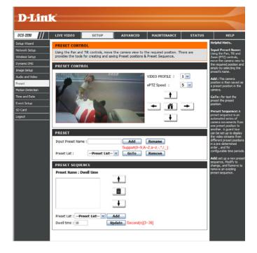
**Preset Sequence:** This section allows you to create a preset sequence, which automatically moves the camera's view between a set of preset views.
