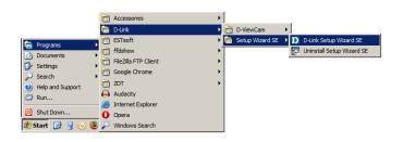
The Setup Wizard will appear and display the MAC address and IP address of your camera(s). If you have a DHCP server on your network, a valid IP Address will be displayed. If your network does not use a DHCP server, the network camera's default static IP address 192.168.0.20 will be displayed.
