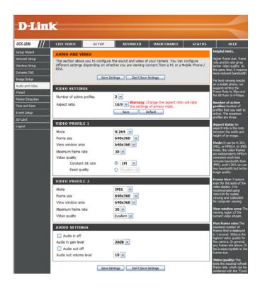
Video Quality: This limits the maximum frame rate, which can be combined with the "Fixed quality" option to optimize the bandwidth utilization and video quality. If fixed bandwidth utilization is desired regardless of the video quality, choose "Constant bit rate" and select the desired bandwidth.
