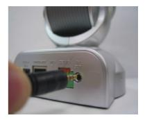
Attach the red RCA connector to the "video" connector on your TV.
