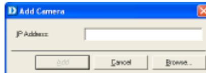
Enter the IP Address of the camera in the specified field and click **Add**. If the IP Address is entered incorrectly or if you have a bad network connection, a dialog box will appear to notify you of the error. To add cameras in IPView Lite, check that you have your network configured correctly. To add a remote camera, you need to have Internet access.
