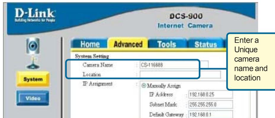
The screenshot shows the D-Link DCS-900 Internet Camera configuration interface. The 'Advanced' tab is selected, and the 'System' button is highlighted. The 'System Setting' section contains the following fields:
