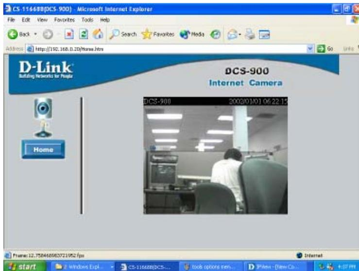
**Camera Name** - The Camera name will be displayed in the top bar located above the camera image when the Camera Name field is entered in the Web Configuration setting under **Advanced > System**.
