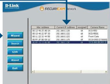
You must change the **Admin ID** and **Password** immediately to protect your camera against unauthorized access. By default, the Admin ID and Password are blank. To change the Admin ID and Password, select both **Change** boxes and enter a **New ID** and **New Password**.
