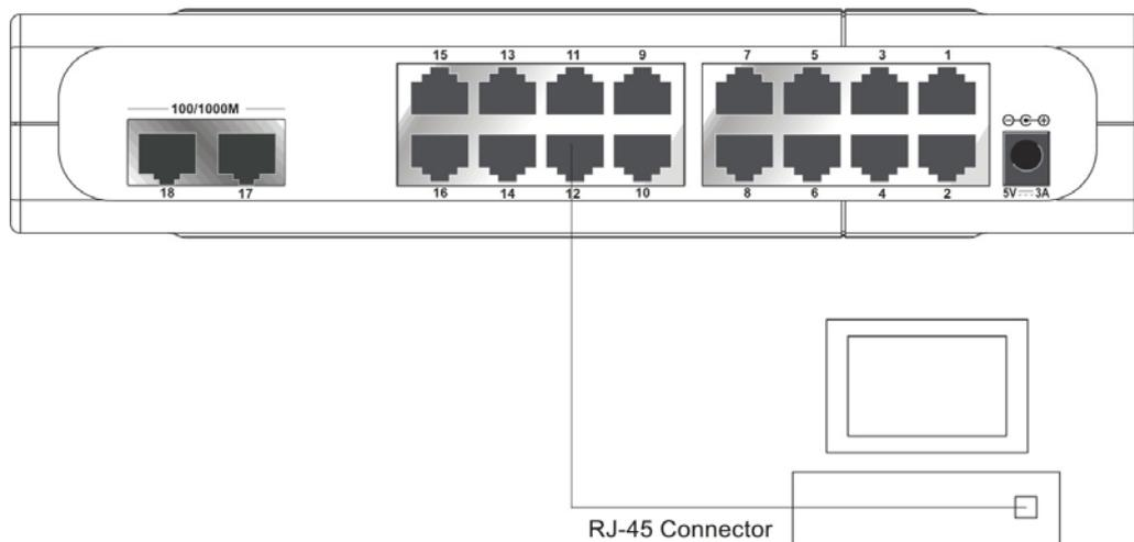
**Figure 3-1. Switch connected to an end node**
