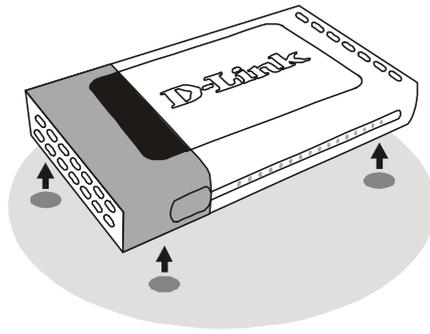
**Figure 2-2. Attaching the Rubber Feet**
