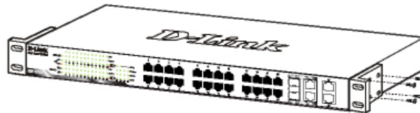
Figure 2. Attaching the mounting brackets
