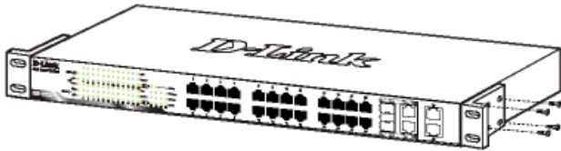
Figure 2 – Attach the mounting brackets to the Switch
