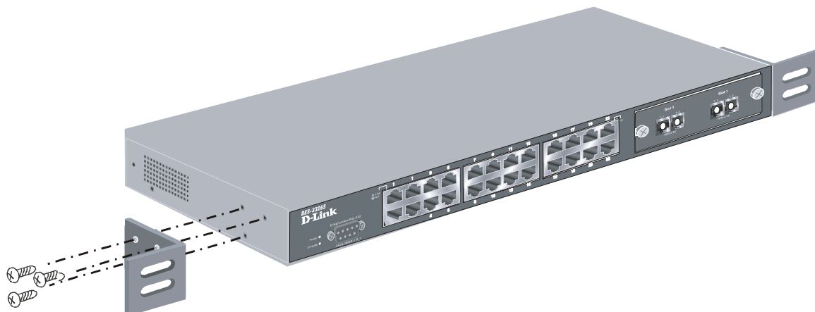
Figure 2-2. Attaching the mounting brackets to the Switch
