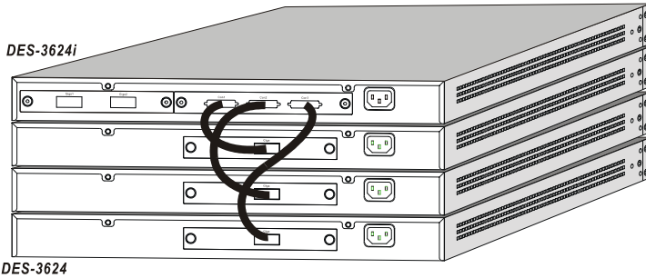
Figure 3-4. Switch stack with one master and three clients
