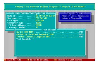
In the Controller Loopback test, test signals are generated at the rate of 100Mbps, and are intercepted and reflected at the MAC level without reaching the network cable.
