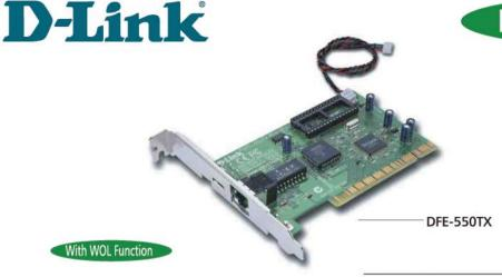
DFE-550TX 10/100Mbps adapter featuring Wake-On-LAN and other advanced functions for direct connection of high-powered PCs to LAN switches and routers.
