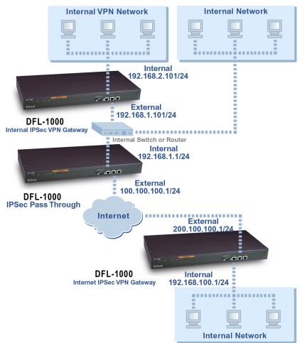
Use the following procedures to configure the internal IPSec VPN gateway, the Internet IPSec VPN gateway, and the DFL-1000 that will be passed through.
