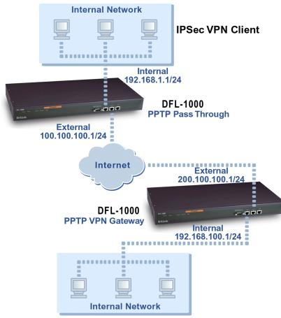
PPTP client connecting to a VPN on the Internet using PPTP pass through
