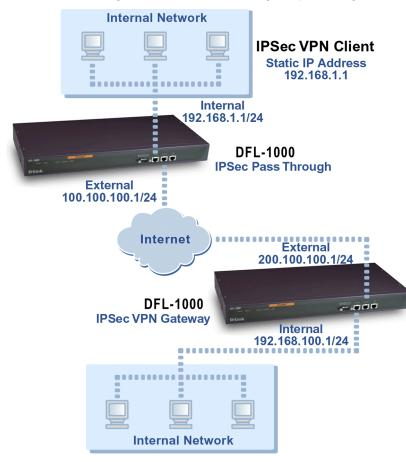
IPSec client connecting to a VPN on the Internet using VPN pass through
