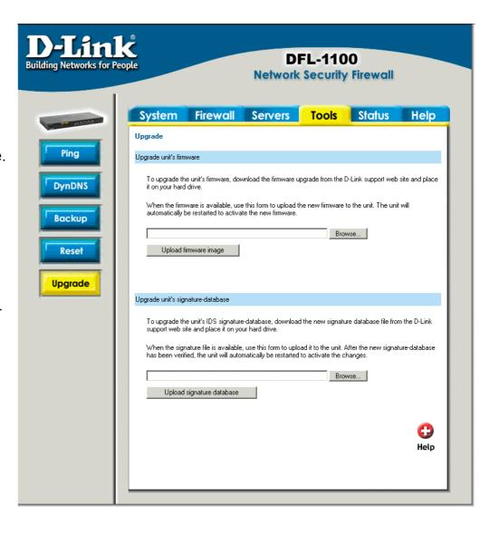
The updating process won't overwrite the system configuration, so it is not necessary but still a good idea to backup it before upgrading the software.
