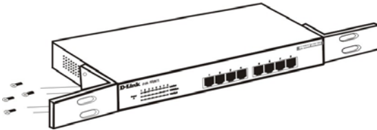
Attaching the mounting brackets to the Switch
