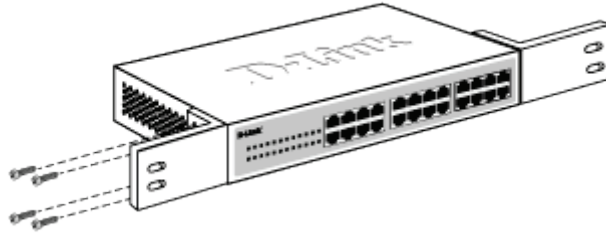
Figure 3-2 – Attach the mounting brackets to the switch
