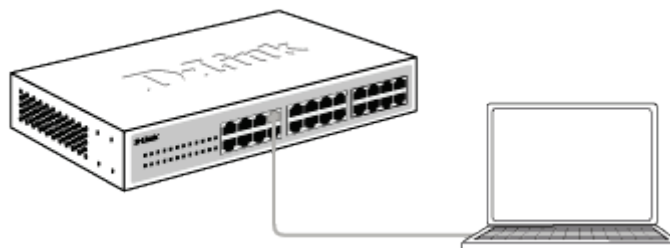
Figure 4-1 – Connecting to a DGS-1100 MP/MPP Series switch
