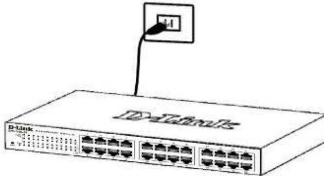
Figure 3-4 – Plugging the switch into an outlet
