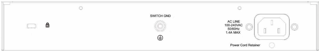
Figure 2-6– DGS-1100-24PV2 Rear Panel
