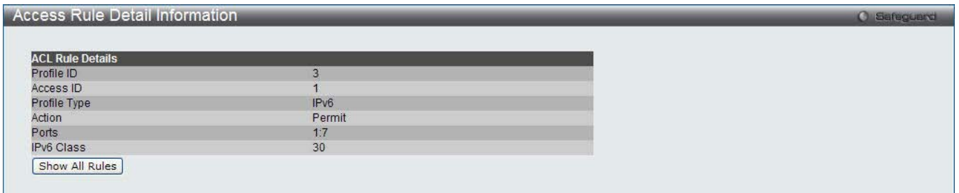
Figure 7-17 Access Rule Detail Information (IPv6 ACL)
