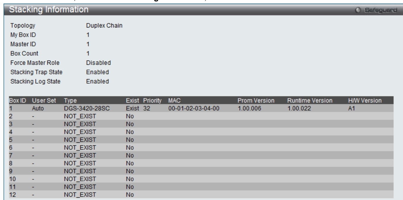
Figure 12-4 Stacking Information window
