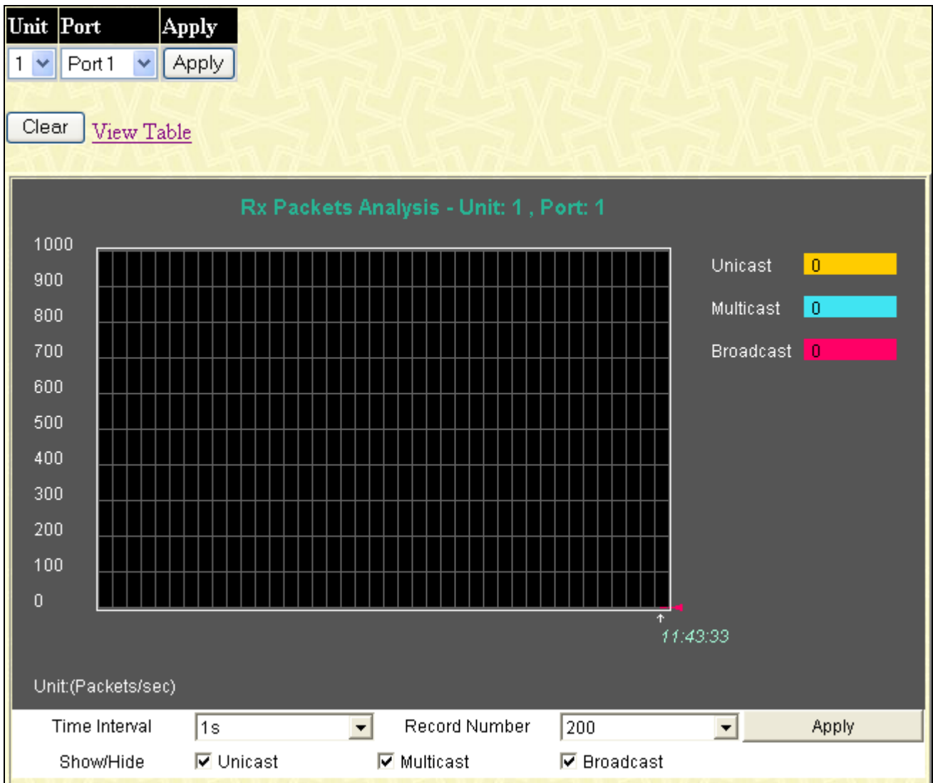
Figure 12- 8. Rx Packets Analysis window (line graph for Unicast, Multicast, and Broadcast Packets)
