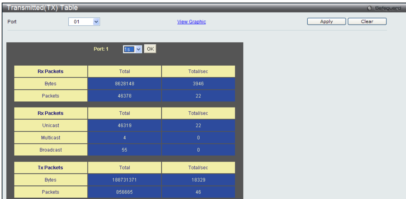
Figure 7 - 13 Transmitted (TX) Table window (for Bytes and Packets)
