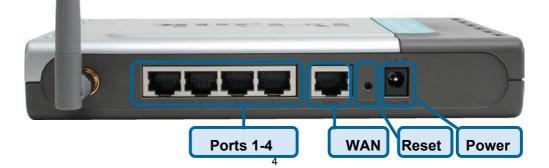
**Reset:** Used to restore the DI-614+ to the factory default settings
