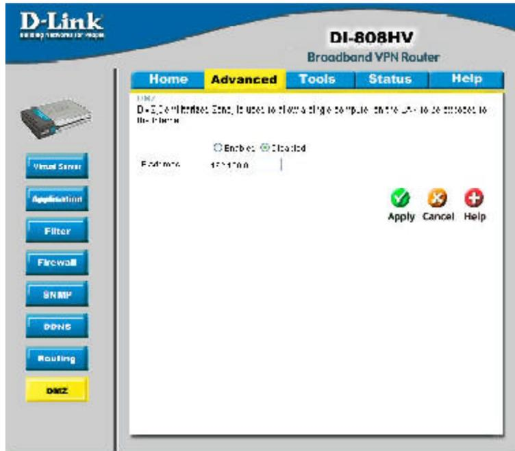
If you have a computer that cannot run Internet applications properly from behind the DI-808HV, then you can allow that computer to have unrestricted Internet access. Enter the IP address of that computer as a DMZ (Demilitarized Zone) host with unrestricted Internet access. Adding a client to the DMZ may expose that computer to a variety of security risks; so only use this option as a last resort.
