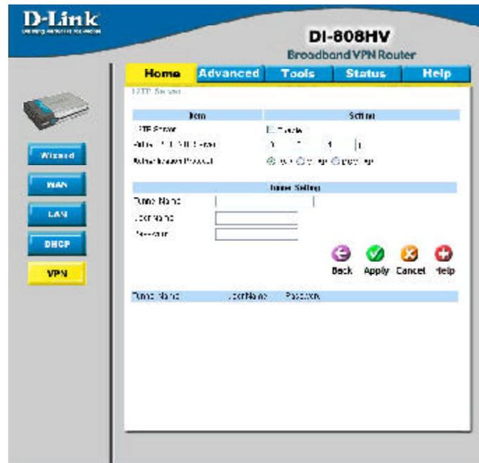
**Enable L2TP Server** Click to enable the L2TP Server function.
