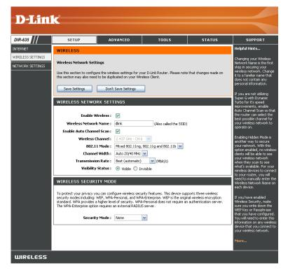
Visibility Status: Select Invisible if you do not want the SSID of your wireless network to be broadcasted by the DIR-635. If Invisible is selected, the SSID of the DIR-635 will not be seen by Site Survey utilities so your wireless clients will have to know the SSID of your DIR-635 in order to connect to it.
