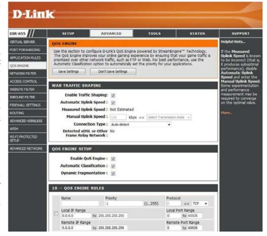
Connection Type: By default, the router automatically determines whether the underlying connection is an xDSL/Frame-relay network or some other connection type (such as cable modem or Ethernet), and it displays the result as Detected xDSL or Frame Relay Network.
