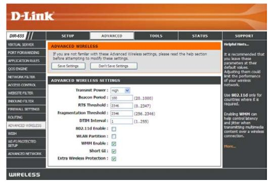
802.11d: This enables 802.11d opration. 802.11d is a wireless specification developed to allow implementation of wireless networks in countries that cannot use the 802.11 standard. This feature should only be enabled if you are in a country that requires it.
