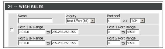
Host IP Range: The rule applies to a flow of messages for which one computer's IP address falls within the range set here.
