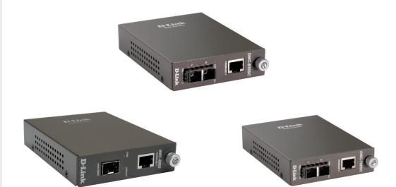
DMC-700SC Media Converter: This converter converts 1000BASE-T Gigabit twisted-pair signals to 1000BASE-SX Gigabit multi-mode fiber signals. The maximum fiber cable distance is 550 m. One RJ-45 twisted-pair port and one fiber port (SC type connector) are provided.
