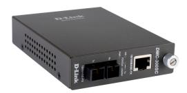
These converters convert 10/100 Mbps 10BASE-T/100BASE-TX Fast Ethernet twisted-pair signals to 100BASE-FX Fast Ethernet multi-mode fiber signals. The maximum fiber cable distance is 2 km. One RJ-45 twisted-pair port and one fiber port are provided.
