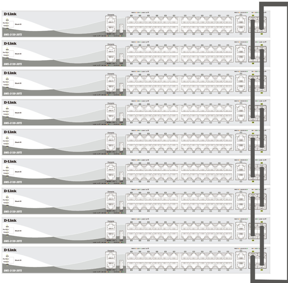
Figure 4-69 Duplex Ring stacking topology (SFP28 ports)
