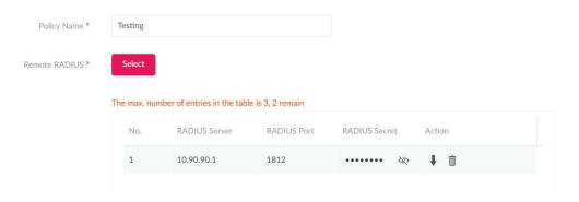
In the **Access Policy Type** field, select 802.1x Port Based. This will allow only one user to be authenticated per port by a remote RADIUS server.
