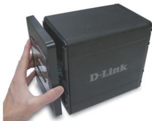
3. Insert a 3.5" SATA hard drive into an available drive bay. Make sure to align the drive connector to the endpoint in the DNS-343. Gently push the drive in until it connects. Repeat for each drive you are placing in the DNS-323.
