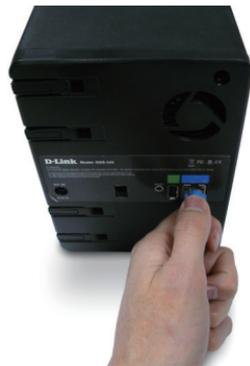
6. Finally, connect the supplied power adapter to the power receptacle on the back of the device.
