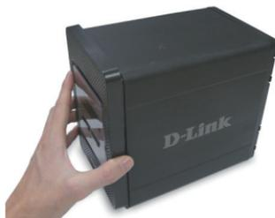
2. Once the faceplate is unlatched, pull it off of the device, exposing the drive bays.
