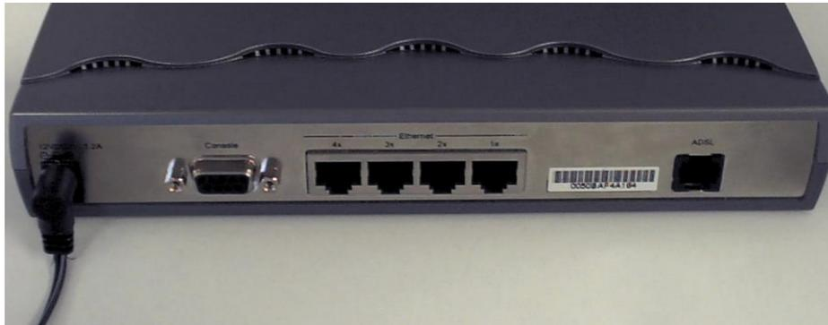
Once the unit power is on, connect one end of the included Ethernet cable to the DSL-504 Ethernet port and connect the other end of the cable into the NIC which is installed in your computer.
