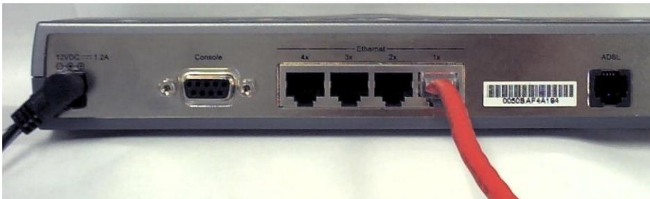
If the cable connection is good, a green LED on the front of the DSL-504 labeled Ethernet/Link will glow steadily.
