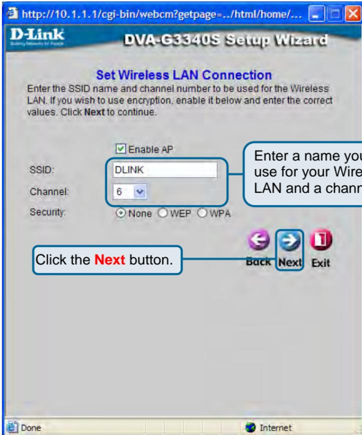
Enter the **SSID** (Wireless Network Name) and **Channel** number you would like to use for your Wireless LAN. ***We strongly recommend that you enable the security feature to keep unwanted users off your Wireless LAN.***
