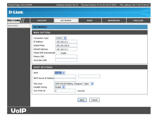
Connection Type: Select DHCP as a network connection to allow the network administrator to distribute the IP address when the gateway is plugged into a different network.
