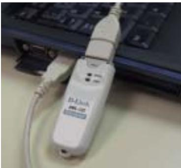
**A.** Insert one end of the USB Adapter into the provided USB cable and plug the other end into your computer's USB Port.
