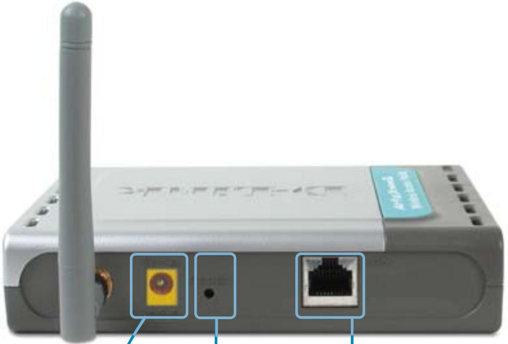
Receptor for the **Power Adapter**
