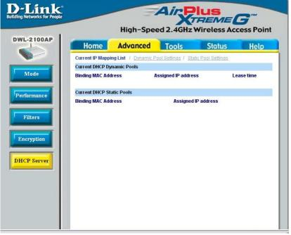
This screen displays information about the current DHCP dynamic and static IP address pools. This information is available when you enable the DHCP function of the DWL-2100AP and assign dynamic and static IP address pools.
