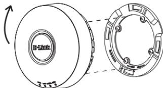
6. Twist counterclockwise to lock the Access Point onto the ring. The lock symbol on the Access Point must point directly to the **Close** text on the mounting ring.
