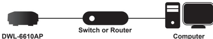
3. Connect the Access Point to a Unified Wireless Switch or Wireless Controller. Connect your computer to the same network as that of the Unified Wireless Switch or Wireless Controller. Manage the Access Point from the computer via the Unified Wireless Switch or Wireless Controller.
