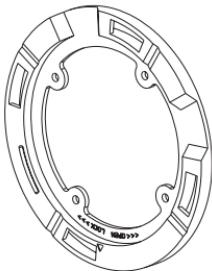
2. Mark the points where you will insert the screws. Take out the mounting ring.
