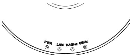
**5 GHz** – When this LED is lit, the Access Point is operating at 5 GHz. It will blink when there is wireless traffic.
