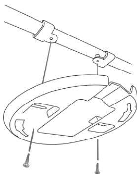
3. Place the DWL-6610AP's male bracket in the mounting ring's female bracket. Rotate the DWL-6610AP clockwise to lock it in position.
