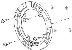
5. To attach the Access Point to the mounting ring, first locate the right side of the Access Point that has a small lock symbol on it, and make sure to line up this side with the side of the mounting ring that has Open - Close written on it.
