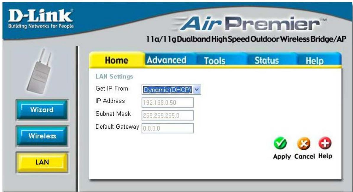
**Get IP From:** Dynamic (DHCP) is chosen here. Choose Dynamic IP Address to obtain an IP Address automatically from a DHCP server in your network.
