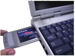
C. Gently insert the DWL-G650 into the Cardbus slot in your laptop computer (as shown.)
