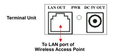
Finally, insert one end of the DC 5V Power Cable that is provided into the Terminal Unit, and the other end into the DC 5V/1A of the Wireless Access Point. The green LED of the Terminal Unit should light up.
