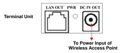
At this point, your Wireless Access Point should have power and function normally. (See the back page of this guide for an illustration of the connected network.)
