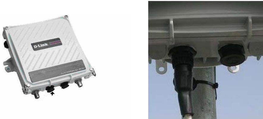
Figure 11. Connect Ethernet cable to Ethernet port
