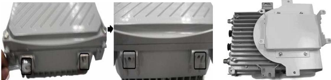
Figure 5 Remove the protectors and slide DWR-500 into the solar shade.
