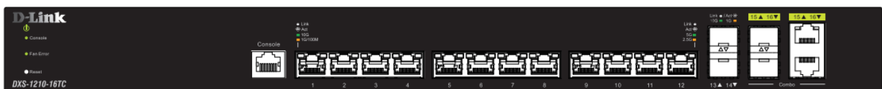
Figure 1.7 – DXS-1210-16TC Front Panel
