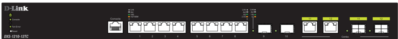
Figure 1.3 – DXS-1210-12TC Front Panel
